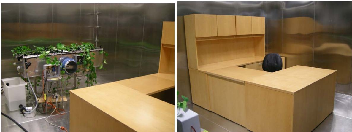
Figure 6 VOCs removal test with real office furniture as the emission source
