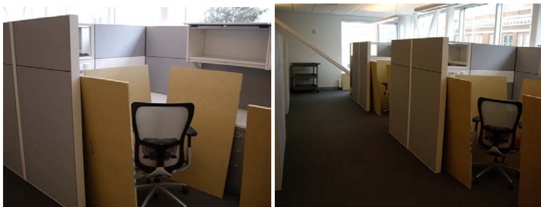
Figure B.1 Contaminant source introduced into the test room by using particleboards
